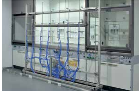
EN 14175-6 type tested fume hood control in acc. with 5.4 Measuring in the outer measuring level
